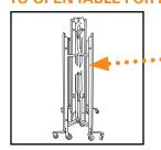
Locate storage latch; pull out to release table from storage position.
