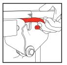
Push down slightly on tabletop while raising the Lock Rod toward the tabletop to release safety lock position.
