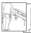
To close, grasp edges of table and pull upward in one continuous motion. Make sure up-latch is engaged.
