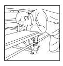
STEP 4A To adjust the Down Latch apply your body weight onto the bench top until the center leg touches the ground, continue applying pressure while completing Step 4B.
