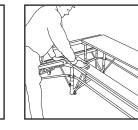
STEP 3 With hands on top of benches, push downward to floor until latch automatically locks into place.
