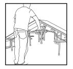
To close, grasp edges of table and pull upward in a continuous motion. Once folded, make sure up-latch is locked.
