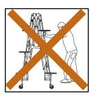
**INCORRECT WAY** Pushing from flat table side may cause tipping.
