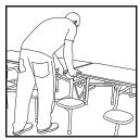
Lower the table to open position until the lock engages.
