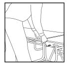
Locate the Lock Rod with one hand and place other hand on table edge
