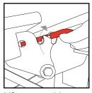
Lift up on tabletop slightly while raising the Lock Rod toward the tabletop to release from safety stop position
