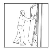
STEP 6 When partially raised, move to center of table/bench and slowly push the table/bench straight into the cabinet so that the table/bench travels squarely into wall pocket.
