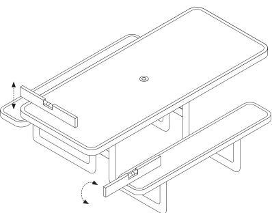
**Note:** Once the table is assembled and the top and seats made level, all hardware should be tightened with tools to 13 lbs-ft.
