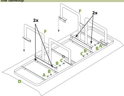
Note: Place top of table upside down on packaging box to protect bench surface when working on the ground.
